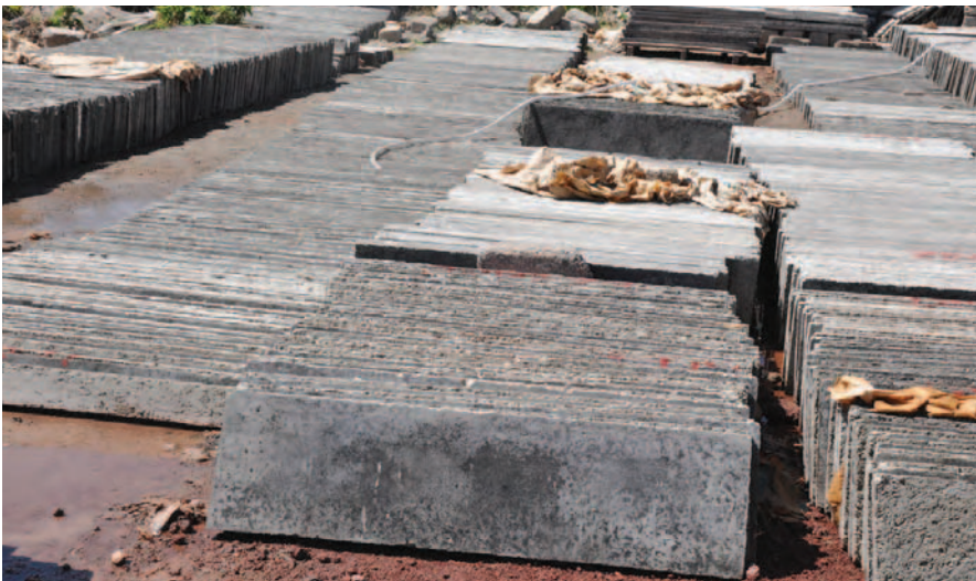
Piles of produced terrazzo tread and window seal
